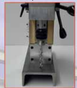
optional with chuck and 19 mm weldon adapter for twist drills
