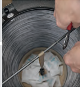
Cut the wire loose
